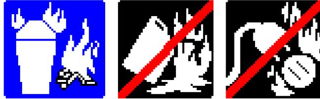
Most fire extinguishers will have a pictograph label telling you which classifications of fire the extinguisher is designed to fight. For example, a simple water extinguisher might have a label like the one above, indicating that it should only be used on Class A fires.
